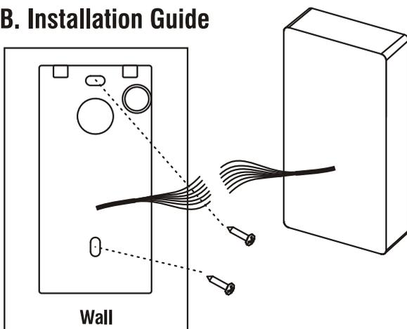
Install back case on the wall and connect cable
